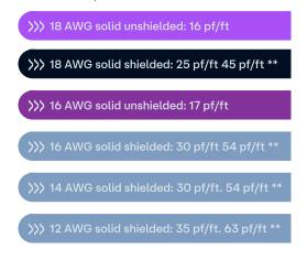
\*\*capacitance between one conductor and the other connected to the shield
