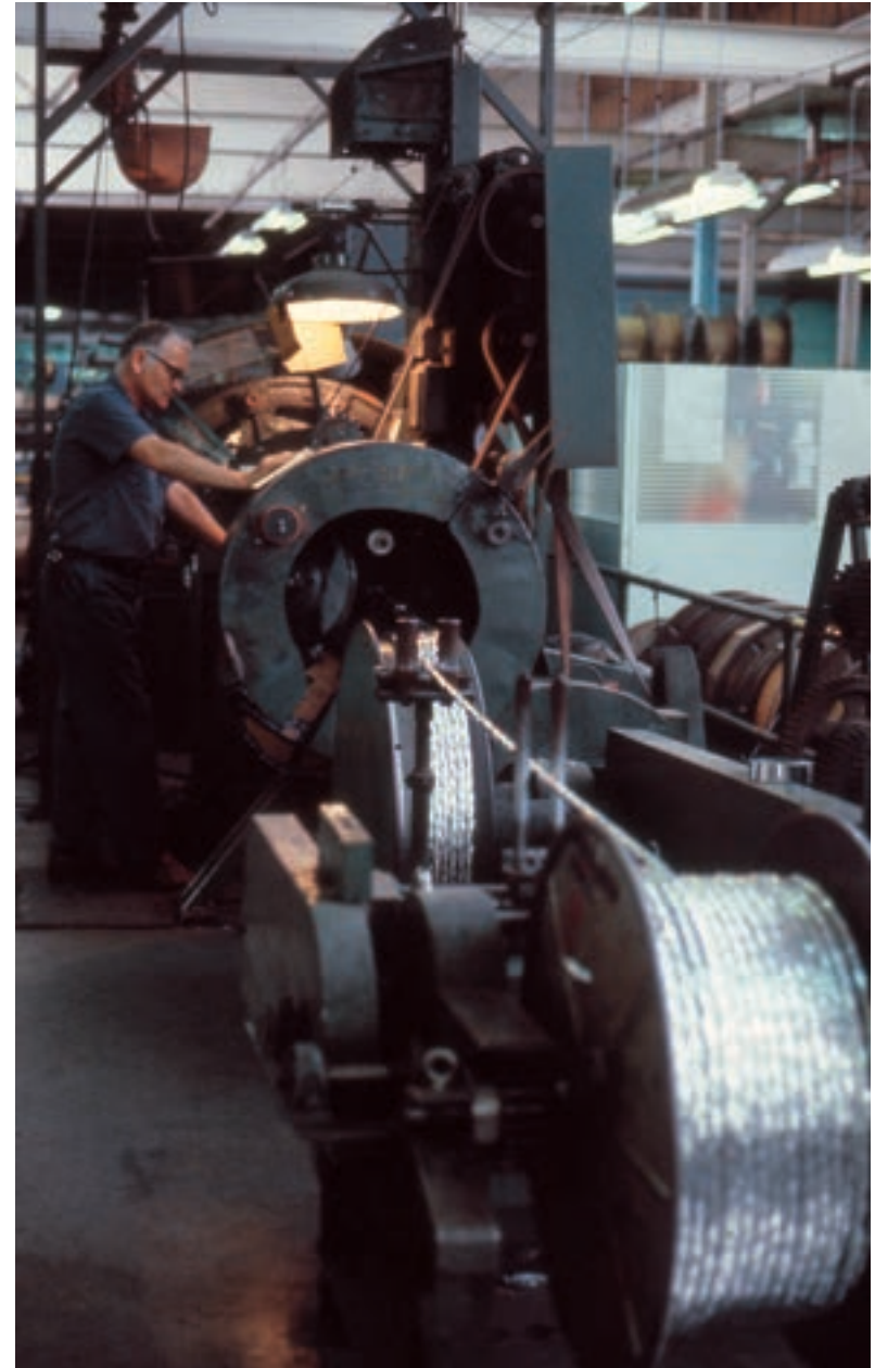
As Belden further penetrated the computer, data and cable TV markets, associates like Bob Mann at the Richmond plant made sure the company's reputation for quality remained excellent; above, Mann applies tape and binder onto cable for jacketing. Opposite, a Belden employee crimps connectors onto stripped wire harnesses.
