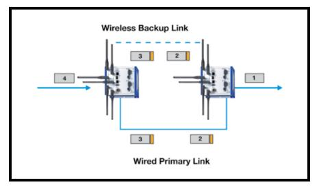
Figure 4. PRP allows both wired and wireless routes to be used as redundant paths, thereby enabling a variety of network topologies. Shown here is a wired path with a wireless backup path.
