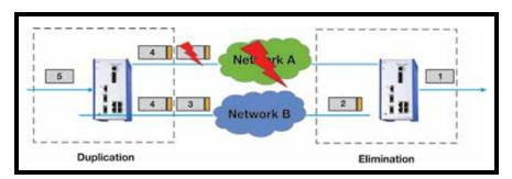
Figure 2. PRP in case of a network failure. Packets from the second network path are used without any resulting switchover times.
