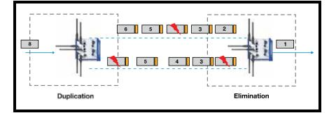
Figure 3. PRP over two WLAN transmission paths: The redundant transmission compensates for packet losses and counterbalances load and interference-related transit time differences.
