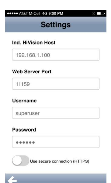
Step 17: Be sure the Apple Device is on a WIFI network and assigned an IP Address on the same subnet as the PC/Server running HiVision.
