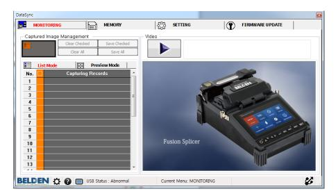
Make sure that the splicer is connected to the computer by USB cable. When DataSync program is being executed, an icon displaying the status of connection to the splicer at the bottom right turns green.
