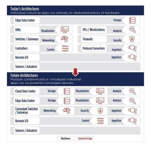
Industrial IoT Edge Architectures Reduce Project Costs and Increase Vendor and Architecture Flexibility through Software-enabled Multi-function Hardware (Source: Belden)
