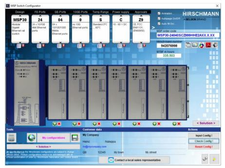
Use the right and left arrow symbols on the parameter selection boxes to toggle the display between parameters 1 to 7 respectively 7 to 13.
