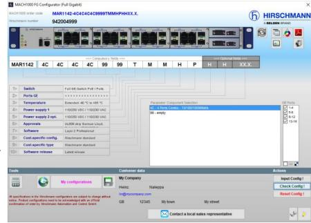
The < Check Config! > button checks your configuration and an advisory message reports possible errors. Once all parameters have been set correctly, the order code and the Hirschmann order number appear above the picture. Additionally the switch is "turned on" which is visualised by flashing LEDs.
