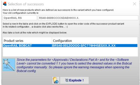
Click on the **Explode!** > button, or double-click on the entry in the list, and the window of the successor will open parallel to the current configurator window.
