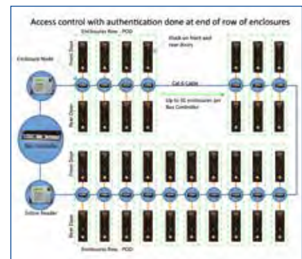
Access control with authentication done at end of row of cabinet
