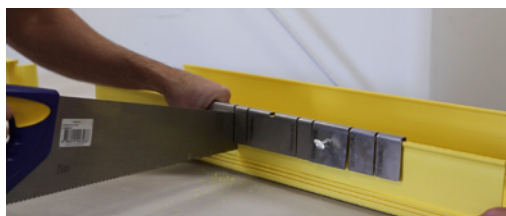
EPN: FRTC1 Cut-out Jig for all ducts.
