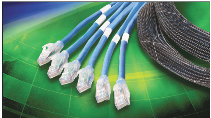
The use of a high-strength braided sleeve serves to protect the assemblies during pulling and routing installation procedures. Cable ends are terminated with RJ45 plugs that are protected with compact and flexible strain relief boots.
