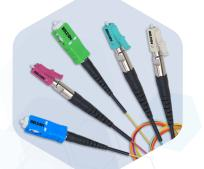
Belden's Fiber*Express* (FX) Fusion Splice-On connectors combine the benefits of fusion splicing with the simplicity of a field-installable connector to expand your options for field termination and improve installation performance and reliability over mechanical splice connectors. No crimping, polishing or adhesives are required for termination, minimizing installation errors.
