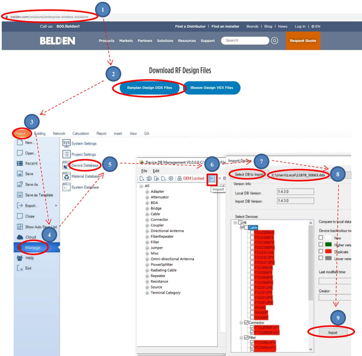
**Figure 2 - Importing Belden Components into Ranplan (Graphical version)**
