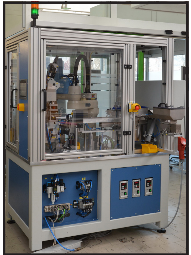
The fully automated robot cell can be moved to any site of operations without modifications, improving efficiency and flexibility.
