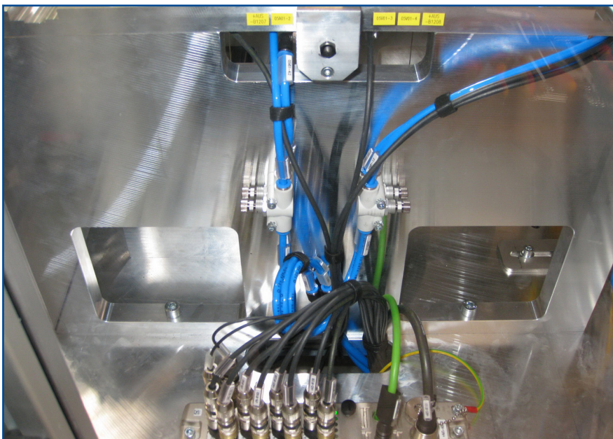
Belden's LioN-R series with vibration and short circuit proof M-12 connectors were selected to meet the challenges of the textile industry.
