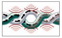
Illustration 1: Example of Non-Bonded-Pair. As cable is stretched and pulled, pairs begin to separate, causing a degradation in signal guality
