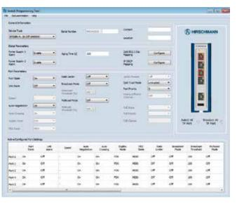
The stand-alone SPIDER Switch Programming Tool runs without installation (even from a USB drive), allowing for the customization of each individual port to the application's needs
