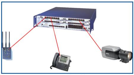
Figure 2.7: PoE endspan power insertion
