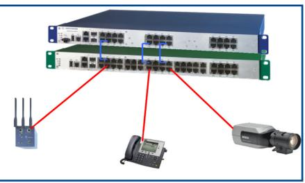
Figure 2.6: PoE midspan power insertion
