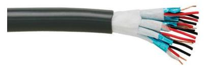
Ideal for general purpose data or machine control applications, the Gepco® Brand HydroBloc™ HBSP series features multiple shielded twisted-pairs under a single round jacket. Each pair is individually shielded and is easy to terminate. With advanced water-blocked construction, the HydroBloc line utilizes a two-ply water-blocking tape and water-swellable fillers to prevent transverse and longitudinal water ingress.
