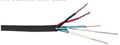
The ABS Type approved 18/22CRTSB cable provides the communications network for multimedia controls in a Low-Smoke, Zero-Halogen (LSZH) construction. Its 22 AWG shielded pair construction with high-grade, low-loss dielectric can serve as a communications circuit while the 18 AWG unshielded pair can power low-voltage devices.
