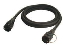
V-CON terminated cable assemblies offer an extremely rugged, compact and weather-resistant portable interconnect system for HD or component video applications. Built with the Gepco® Brand V-CON connector and Gepco Brand multi-channel video snake cable, V-CON cable assemblies can be custom ordered in three- to 16-channel versions.
