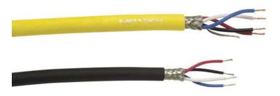
The MP1201 and MM1024 microphone cables use the industry-proven, quad-star design and tight-angled, full-coverage braid shield for maximum low-frequency EMI noise rejection. Four conductors form a "double balanced" system that minimizes the loop area and reduces noise induction from external sources such as AC lines and dimmer packs. As a result, this series is ideal for applications where high EMI is present or where a redundant pin-to-pin connection is desired for improved flex-life.
