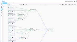
Node-RED based flow editor for manipulating and visualizing OT and IT data
