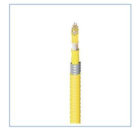
Belden's tight-buffered multi-fiber distribution cables are available in fiber counts from 2 to 144. These highly popular cables are designed for both indoor & indoor/outdoor applications. Distribution cables are available in plenum, riser, unitized & non-unitized constructions which fit a wide array of general purpose installations. Their small bend radius and 900µm tightbuffered fibers allow for fast installations and easy terminations.
