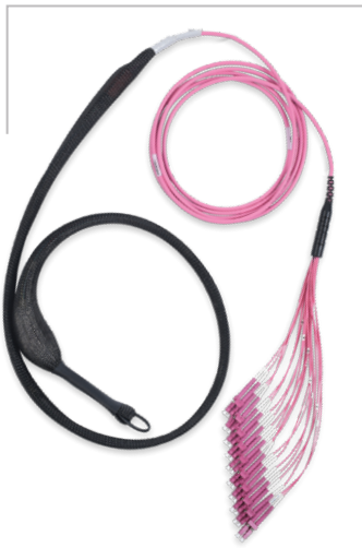
TL Harness, Kit TLX1280 (Top), OM4, 4 x Trunks (fill one card), LC Duplex (1.6 mm x Staggered) - LC Simplex (900 μm x 1.0 m x In-Line), OFNP, 10 m, Erika Violet Jacket
