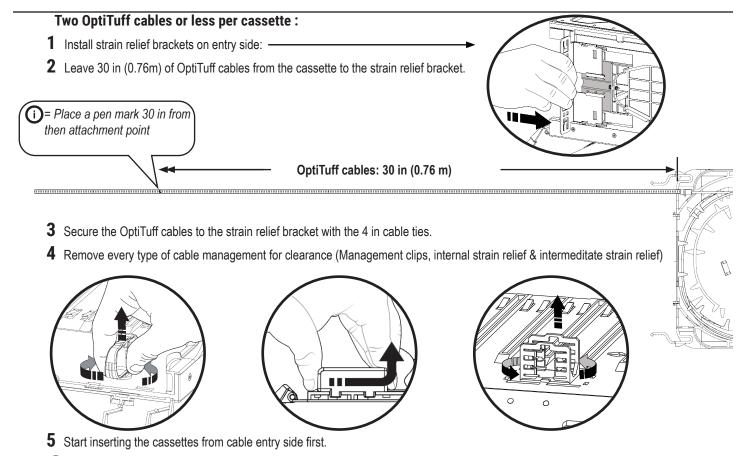
(i) = Make sure the cables enter through the top of the cassettes, whether your cable entry is top or bottom, left or right.
