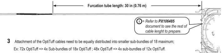
3.1 Prepare each sub-bundles and secure by tightly wrapping a cable tie (4 in cable tie) on the Heat shrinked OptiTuff portion.
