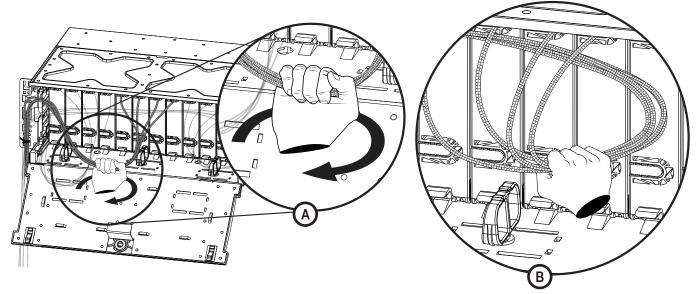
8.2 Place the bottom portion of the loop into the indicated management clip.
