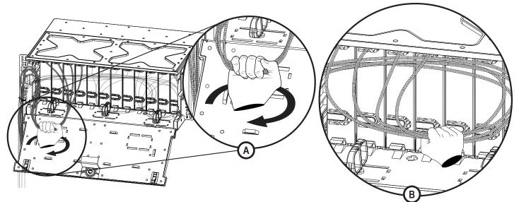
9.2 Place the bottom portion of the loop into the 2 indicated management clip.
