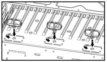
7 To cable manage this OptiTuff configuration, start routing the 4 cassettes farthest away from your cable entry.
