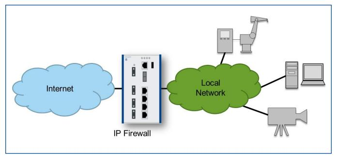
Fig. 1: Firewall between the Internet and the local company network
