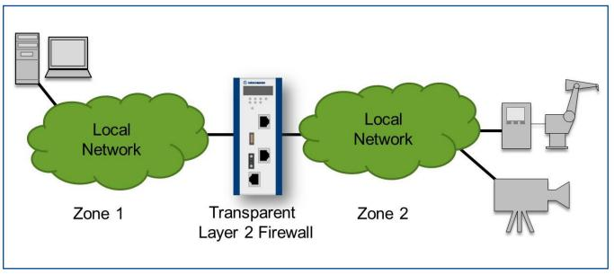
Fig. 2: Firewall within a local network
