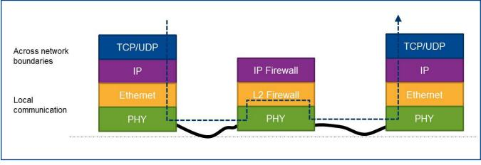
Fig. 3 - Layer 2 transparent firewall
