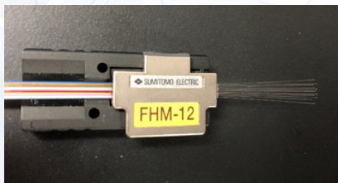
Figure 8: Properly Straightened Fibers
