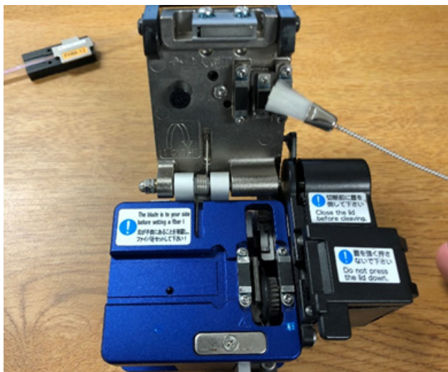
Figure 9: Clean Contact Pads in Cleaver
