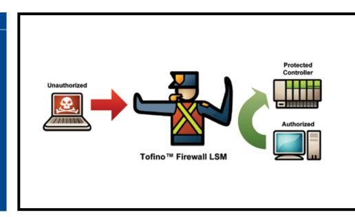
The Tofino Firewall LSM is like a traffic control cop for industrial networks, checking all communications on your control network against a list of traffic "rules" defined by your control engineers.
