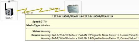
Therefore the data throughput is maximized. Over time, the antennas may become misaligned, usually as a result of harsh weather, such as strong winds. In this case, the data throughput deteriorates progressively, until the link fails entirely.
