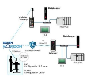
This type of remote connection is for a specific purpose. Examples include checking status, changing PAC software, or upgrading firmware. The user will disconnect once the action has been completed.
