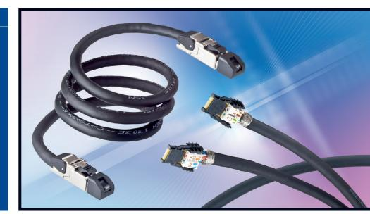
Belden® CatSnake™ CAT 6A tested cables deliver superior performance thanks to the 100% coverage of the pairs individually shielded with Beldfoil® aluminium/polyester foil and an overall braided shield.
